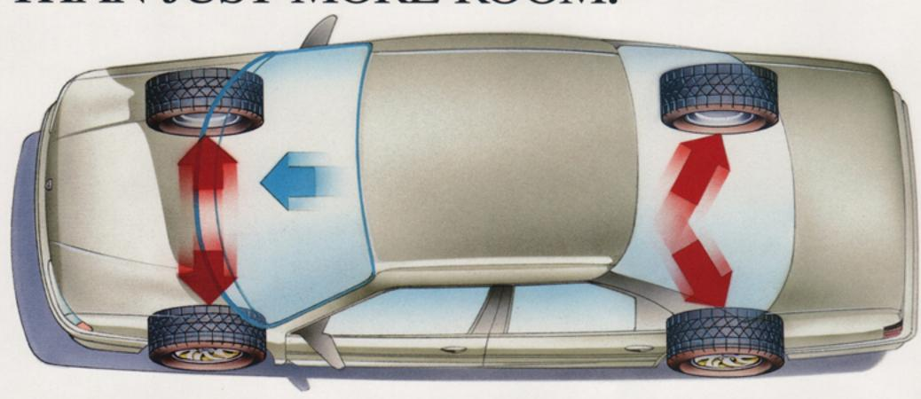
Pushing the wheels toward the corners enhanced stability and handling. Moving the leading edge of the windshield reduced wind noise and increased visibility. It's all part of a revolutionary cab-forward design that makes this car look and feel very different.
